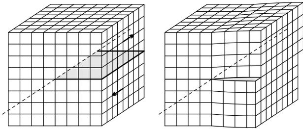
FIG. 2. Volterra construction of a screw dislocation.
