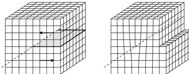
FIG. 1. Volterra construction of an edge dislocation
